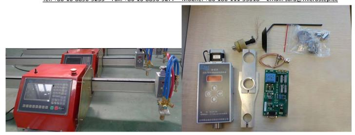
It's also made by us. This model is specially designed for our CNC cutting controllers. It can automatically adjust the height between the torch and plate. Now more and more CNC cutting machines use the torch height controller, especially for plasma cutting. Most clients buy our CNC cutting controllers and torch height controller together to make machines.
